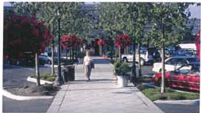
Parking and Access. Parking is prohibited between the front of the building and the street in order to create a more cohesive and continuous pedestrian experience [1] Parking may be located to the side if it does not exceed 50% of the total site frontage [2] Clearly marked, attractive, safe pedestrian paths through parking lots should be provided to reduce conflicts with automobiles.
