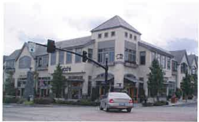
Primary entry located within 25 feet of corner, increased height at the corner with a pitched roof, special pavings and plantings provide public gathering space, articulate a gateway into the district, and provide a means of way finding.
