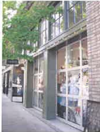
Large glass entry door, large windows, transom windows, columns, and pedestrian oriented signage.
