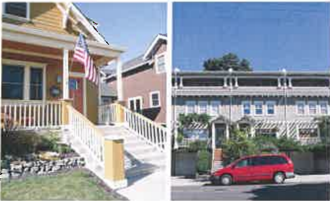
Main Entrance. Buildings should have [1] front doors that face the street and connect to the sidewalk via a 5 foot wide path at a minimum [2] Porches should be an extension of the living space and be at a minimum 5 feet clear in depth.
